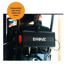
In 2023, CBL introduced 'DROVE' in partnership with Deakin University's Applied AI Institute, an autonomous wheelchair system. Whilst it can be used within CBL's ecosystem, it can also be used independently of CBL's devices. Essentially an add on module for powered wheelchairs not requiring a joystick or wheel to operate, allowing incapacitated users to navigate their homes independently and safely with reduced cognitive and physical strain.
